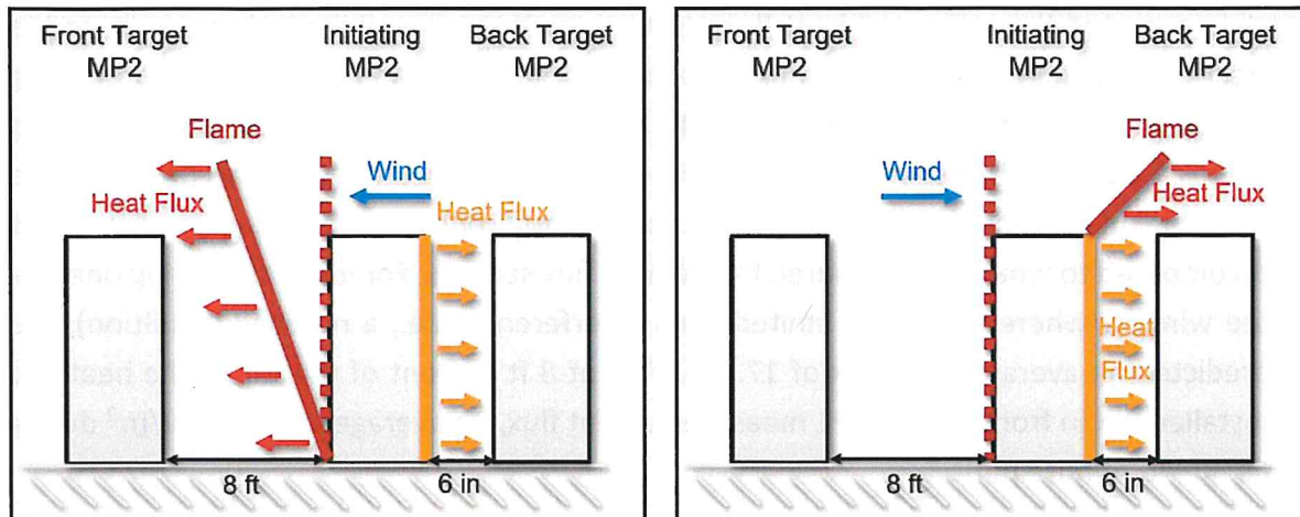
Figure 24 Heat flux model conditions: with wind blowing towards the front target (left) and with wind blowing towards the back target with flames exiting the top of the MP2 cabinet (right). Note: the illustrations are not to scale.
